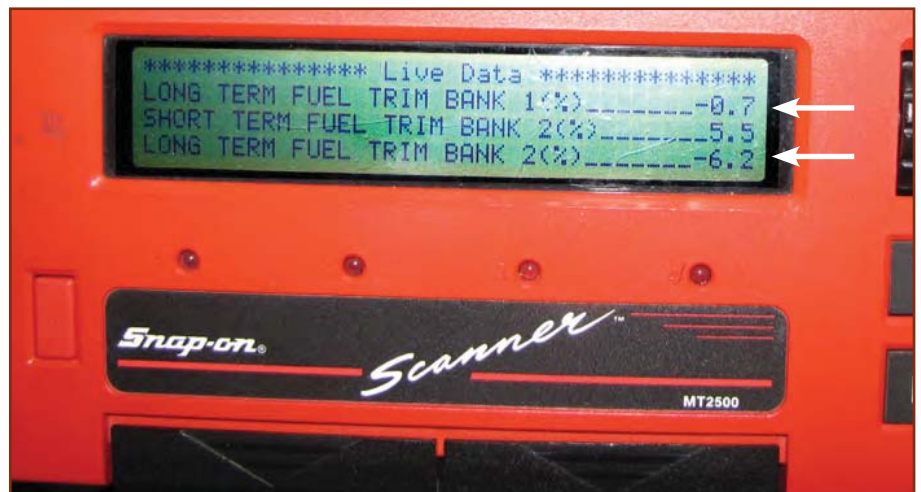
Figure 2a: This vehicle has a v-8 engine and reports bank 1 and bank 2. Notice bank 2 has a large disparity from bank 1, at -6.2. This could be caused by any number of problems: a leaking fuel injector, an O2 sensor, a bad spark plug or spark plug wire etc. But since it's only on one bank it would not be something that would affect both sides, like a MAS or TP sensor.
