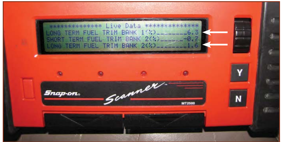
Figure 2b: Here, we've added a vacuum leak and let it idle for about 15 minutes, to illustrate its effect on Long Term Fuel Trim. Long Term Fuel Trim went up 7 points on bank one and 7.8 on bank two. We're a long way from setting any codes but we're getting near that area where drivability problems begin to occur.
