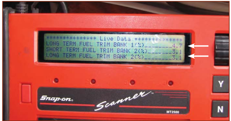
Figure 4: The Fuel Trim reading look normal. The low reading at an idle is worth noting. You may not have any problems now but it's good to note this in case the customer has problems later.
