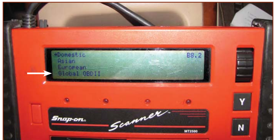
Figure 1: By using the Global OBD II setting your scan tool will display fuel trim the same on every car you check. This'll give you a chance to become familiar with the readings.
