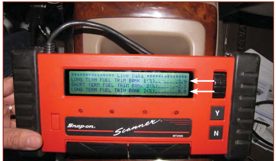
Figure 3: At 1,500 rpm the readings are in range. At a higher rpm that fuel leak has no effect on the system.
